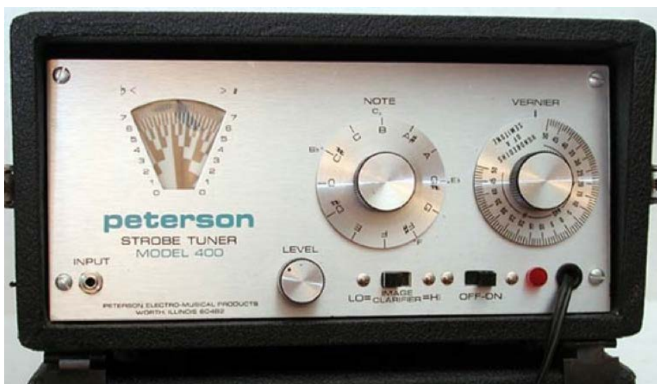
FIGURE 1. Peterson Model 400 stroboscopic tuner (copyright Peterson Electro-Musical Products—licenced for all uses under Creative Commons Attribution-ShareAlike 3.0).
